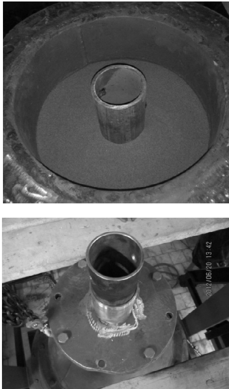
Fig.10. Details of steel model piles driven in FCV with Casing guide
