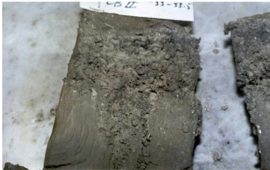
Figure 2: Stained fissures filled by fine sand, by Jakobsen Co [3].
